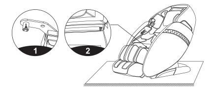
3). Insert the R-shaped pin, move the calf to the other side, and insert the R-shaped pin (Figure
